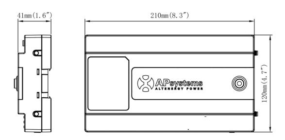
The APsystems Gateway, our state-of-the-art Energy Communication Unit (ECU), is the information gateway for APsystems inverters. It collects and transfers module performance data giving you comprehensive monitoring and control over each individual module, optimizing the performance of your solar array.
